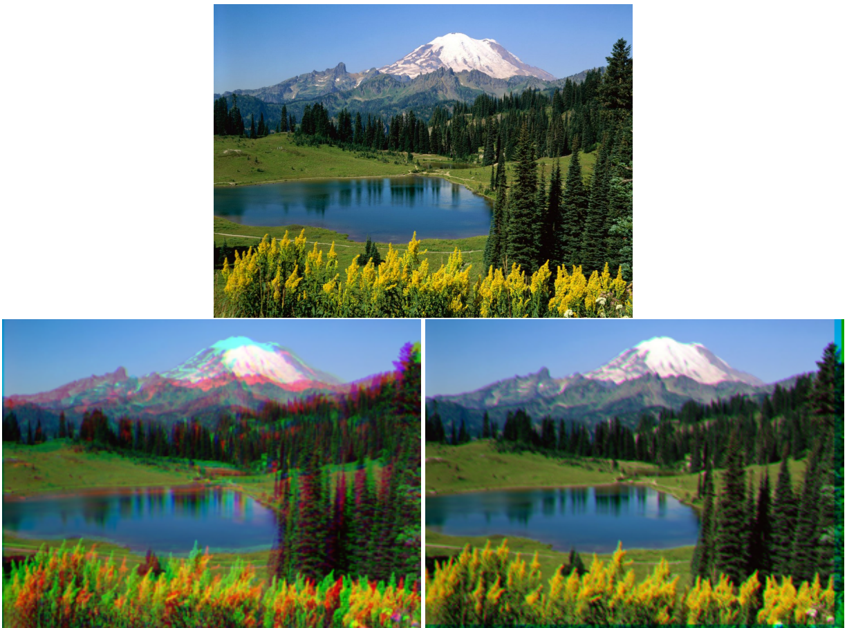
Figure 6: Top: The original image from Google Images. Left: The same image with a different translation shift in two of the colour channels. Right: A corrected version using our algorithm.
